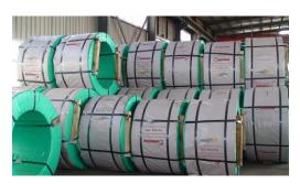
Post-tension (PT) strands are manufactured in accordance to the standard American Society for Testing and Materials (ASTM) A416. It is composed of seven treated carbon steel wires, six of which are arranged in a helical pattern around a slightly larger center
